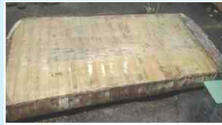
Titan31A forged annealed plate (Finish forging of plate in 6000T press is depicted at the corner)
